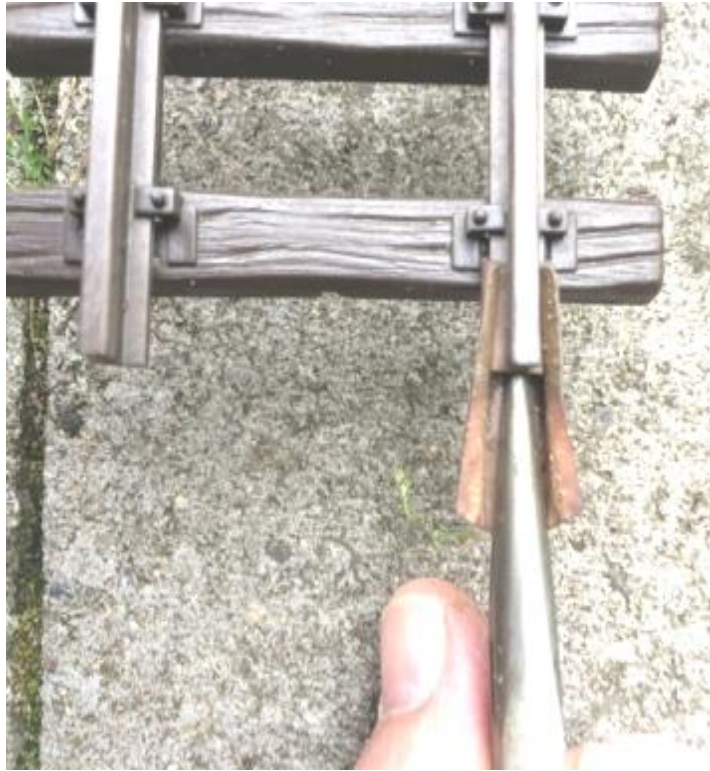
Fig 2.5-14 Bending open an LGB rail connector
