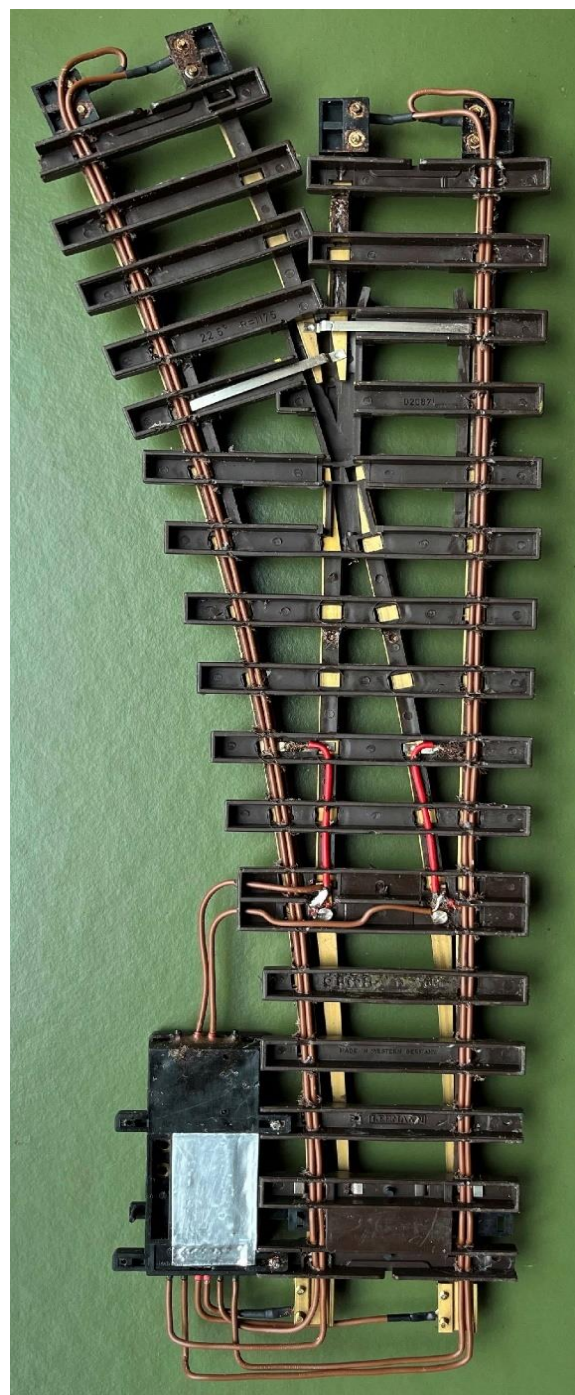
Fig. 2.5-5 The same point seen from below. The two red wires provide better supply of current for the point blades.
