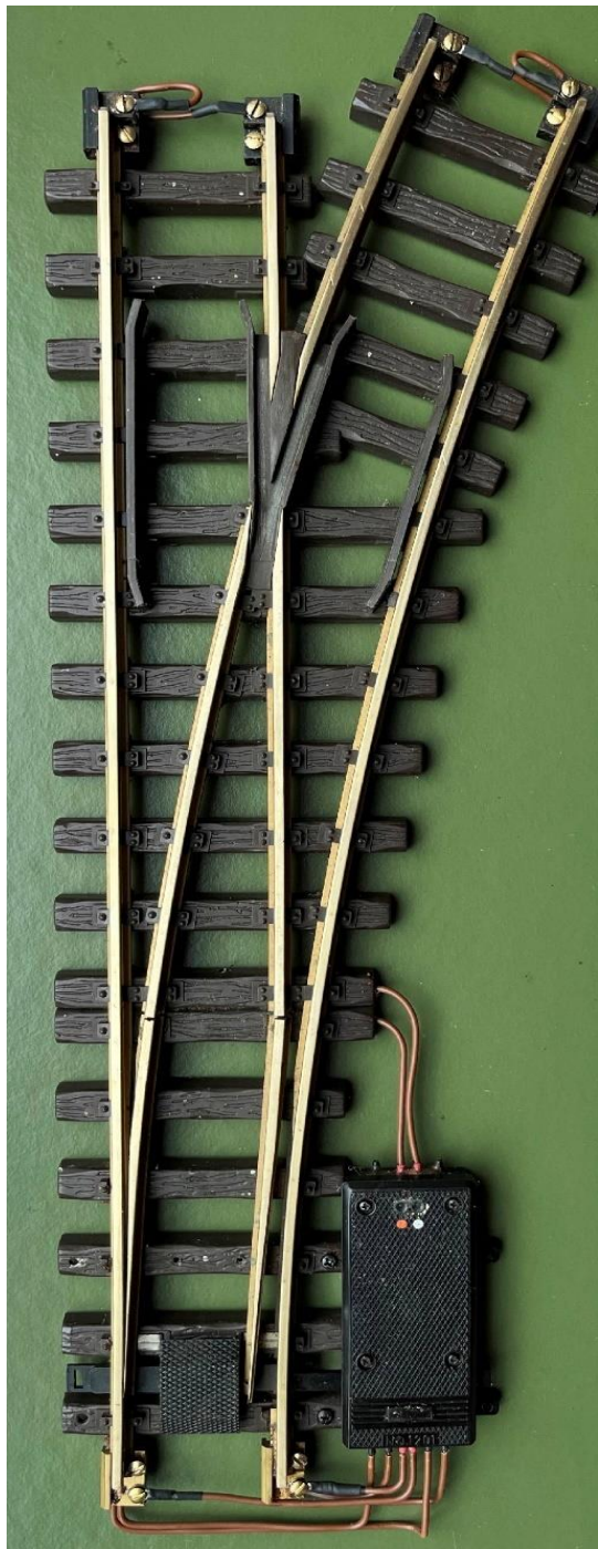
Fig. 2.5-4 Point LGB 16050 with drive and decoder Zimo MX820D and switch contact RBK310610 with built in wiring seen from above.
