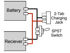
These charging jacks show three connections but for a different reason than the three tab jack shown earlier. This smaller jack only has the two wires attached. The third hole and pin/tab have no wires connected and are only there to keep someone from inserting it incorrectly. When inserted correctly the two wired connections mate. If reversed only one connection is made and no harm is done. By convention the black wire from the battery and charger is connected to the center of the three pins.
