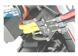
For most O scale and all HO scale this charging jack is too large. It would work but is grossly out-of-scale. In such applications I use a very small plug connection that looks like this. These are made from common 0.1" pin connectors used in the electronics hobby.
