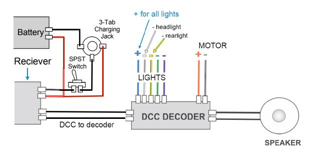
The following diagram illustrates how the various components fit together.
