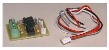
The **#SSI-12v3** replaces the regular **SIERRA**® 6 volt battery & provides an optically isolated motor reference. It is required to access the "At Idle" effects such as the spent exhaust, stop toot & firemen Fred. 33mm x 25mm x 10mm.
