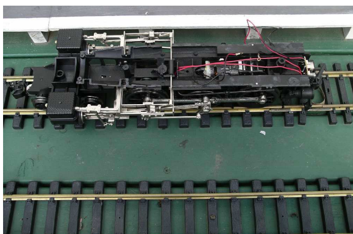
The BTR model of a PB15 loco was modified by undertaking a major kit bashing of a Bachmann Big Hauler.
