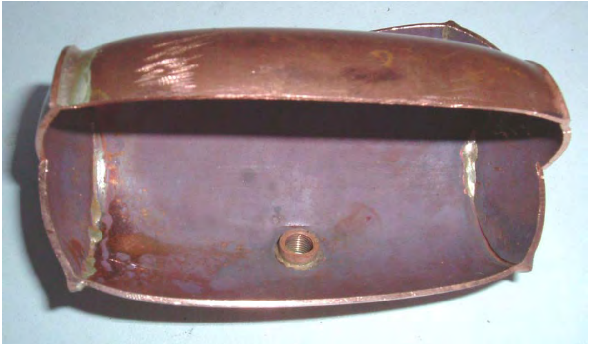
No11 Sectioned. The incomplete solder penetration can be seen on the right hand side of the piece.
