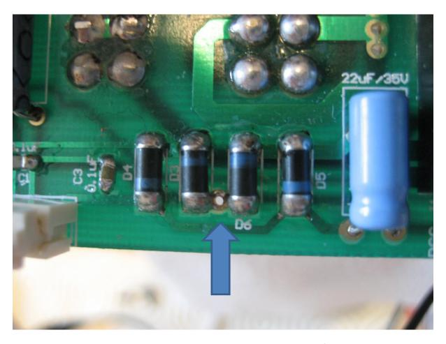
The arrow shows the plated through hole that was intermittent. A piece of wire was inserted and soldered in place. The bad connection has now gone.
