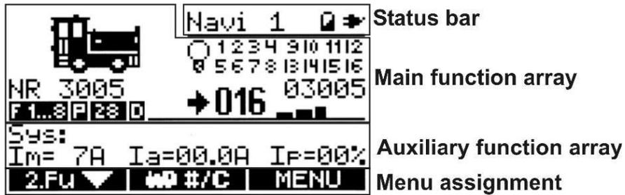
The special functions, like smoke generator, lights, sound functions etc, are operated with the function keys 1...8.
