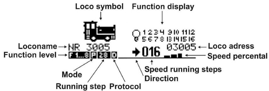
**Selecting the Loco Address** After pressing the locomotive selection key M2 the DiMAX Navigator displays the locomotive selection window. Enter the loco address via the keypad, for example, loco address 0021 After confirming the address by pressing M3, the loco is ready for operation and the DiMAX Navigator automatically returns to the driving mode screen.
